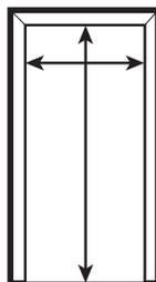
If the opening is less than 80" high: Stack the door panels together, secure with masking tape and cut with a hacksaw or fine tooth saw. Remove the masking tape. Cut the overhead track 1/8" shorter than the width of the opening.
